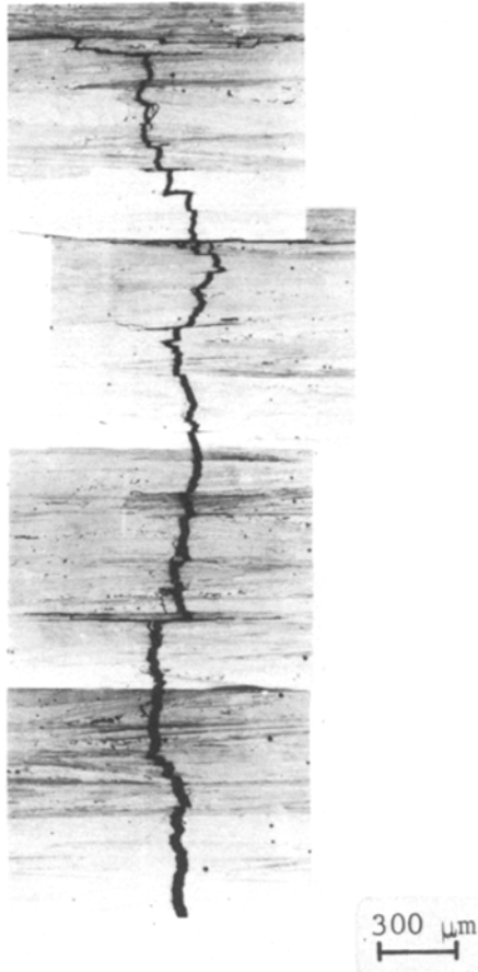
Figure 11 Typical longitudinal fracture surface profile illustrating erratic crack growth and delaminations. Preparation – ET.
